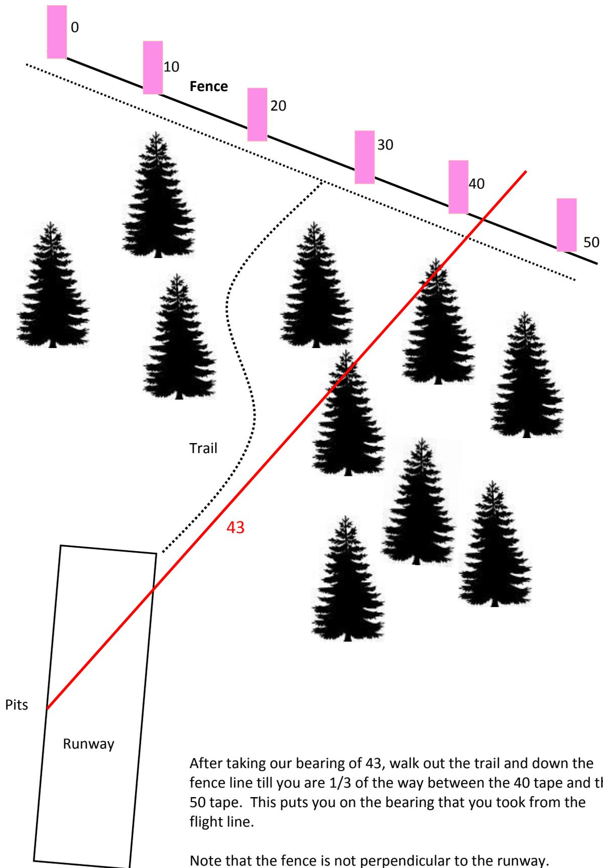
After taking our bearing of 43, walk out the trail and down the fence line till you are 1/3 of the way between the 40 tape and the 50 tape. This puts you on the bearing that you took from the flight line.
