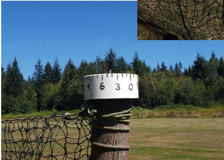
To take a bearing, sight over the top of the pelorus, lining up the centre pin with the object you want a bearing of. In this case the tree top in line with the pin is just a little to the left of the mark which is left of the 3 mark. Each mark is 10 degrees, so the bearing is between 40 and 50. I would call it 43.
